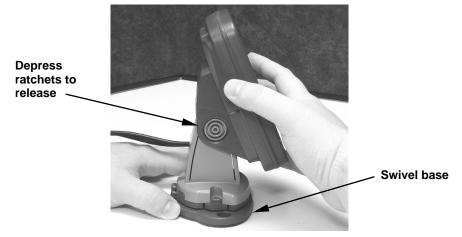
Adjust viewing angle: use one hand to press and release the springloaded ratchets while you move the unit with the other hand.
